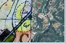
Figure 2: a displacement of 307 meters is seen between the topographic map base for the VTM dataset (a) and the 2005 NAIP imagery used by the NSNF project (b). The displacement measurement measurement measurement and the second seco is between the crossing of Butte Creek by Centerville Road.
