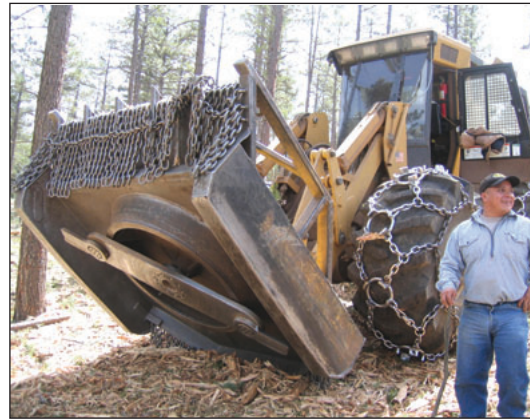
Figure 8. A hydro-axe is used to grind up trees to reduce canopy fuel loads and lower the risk of crown fire. Photo by Dan Binkley, Colorado State University.
